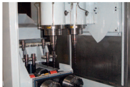
Two spindles DigitalSuper devices with two aerosol generators work with machine centers with two spindles
